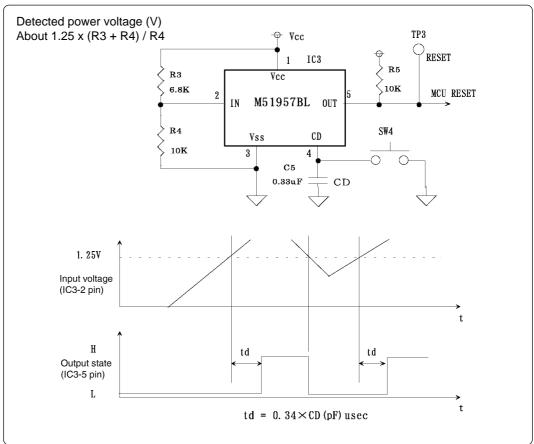
Figure 6.1 Reset circuit and its waveform
